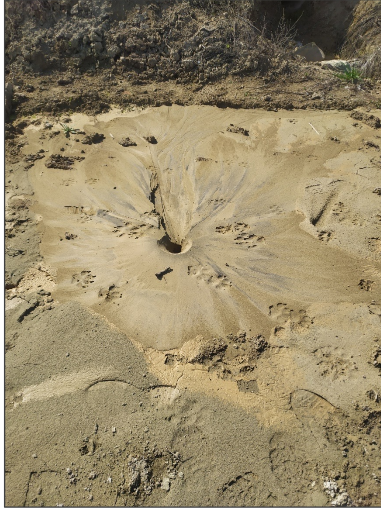
Free-field soil ejecta sites at Demirköprü-Hatay, Kumlu-Hatay and Gölbaşı-Adıyaman after Kahramanmaraş Earthquakes
