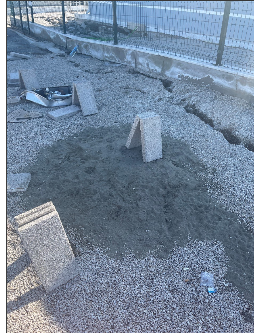
Liquefaction-induced deformations at a private port in İskenderun and Fishery Warf
