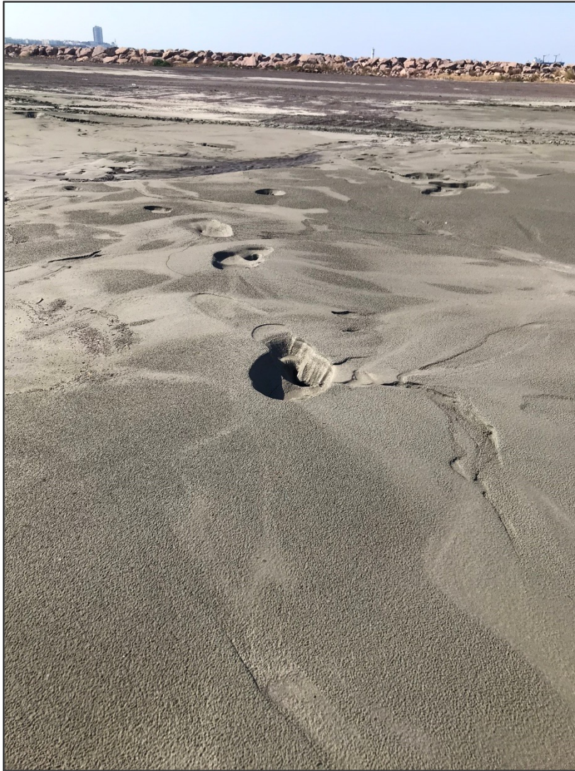
Liquefaction-induced deformations at a private port in İskenderun and Fishery Warf
