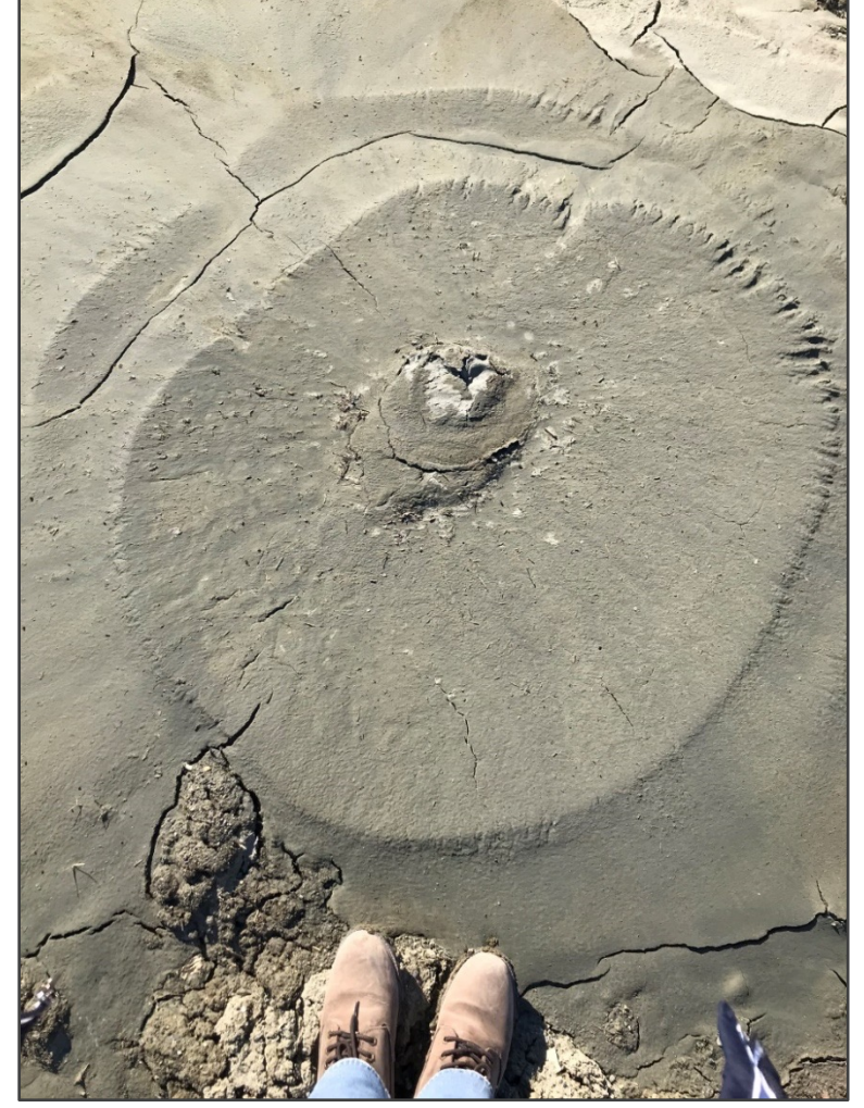
Free-field soil ejecta sites at Demirköprü-Hatay, Kumlu-Hatay and Gölbaşı-Adıyaman after Kahramanmaraş Earthquakes
