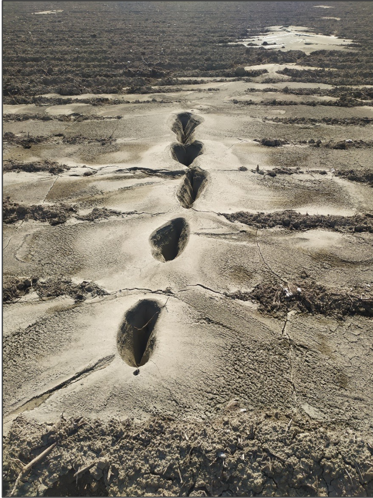
Free-field soil ejecta sites at Demirköprü-Hatay, Kumlu-Hatay and Gölbaşı-Adıyaman after Kahramanmaraş Earthquakes
