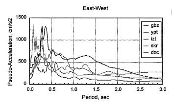
Figure 6 - Response spectra (5% damped): a) north-south components, and b) east-west components. The north-south component in Sakarya was not available. (Records provided courtesy of the Earthquake Research Department of the General Directorate of Disaster Affairs and Bogazici University.)
