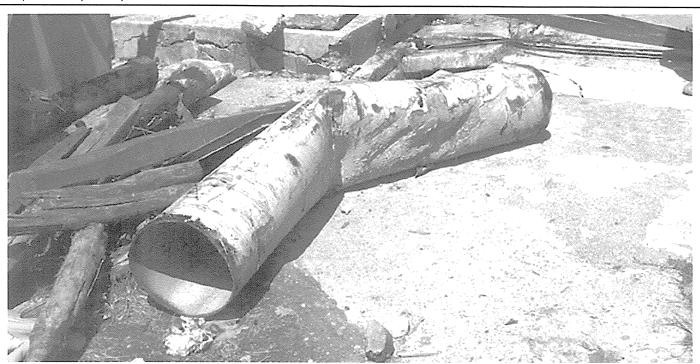
Figure 12 - Buckled steel pipe at crossing near Arifiye.
