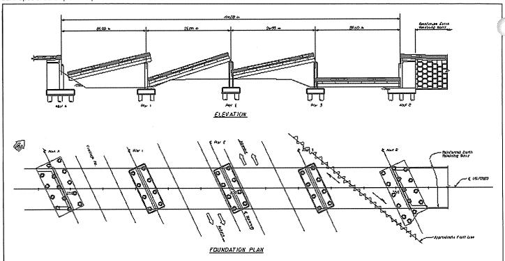
Figure 10 - Plan and elevation of collapsed overpass
