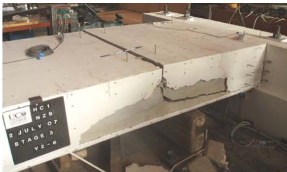
(a) Negative moment flexural failure
