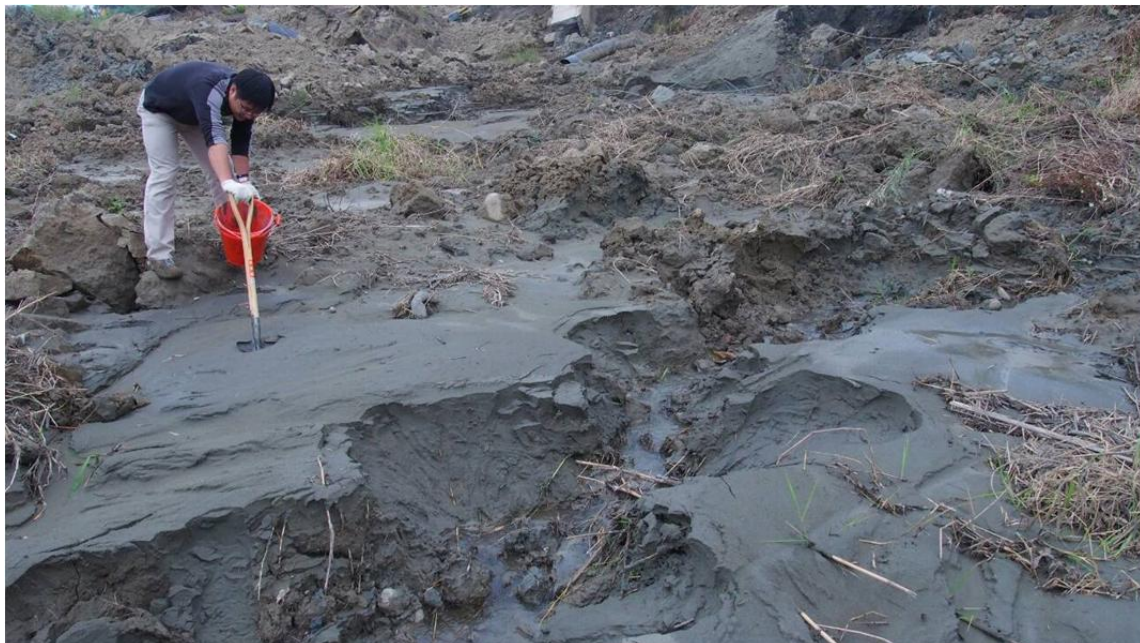
Figure 4.5 Collecting samples of liquefied soil at the lateral spreading site of Zengwun River embankments (provided by Hsuan-Chih Yang)
