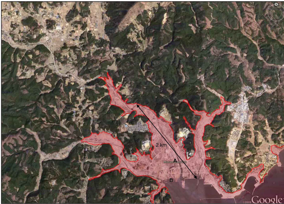
Figure 8. The approximate inundation zone in Minimisanriku Town. The tsunami surges destroyed the town center and went up the narrow Hachiman River (center) and the Sakura River (on left) and the Oretate River (on right). Black arrow is 2 km long. (A) marks the location of the disaster management building shown in Figure 10 and (B) shows the tsunami evacuation building in Figure 26. The gates shown in Figure 9 are just to the right of B. The inundation area shown here (and in Figures 12 and 15) is based on Google earth imagery and may change when data from field teams is included.
