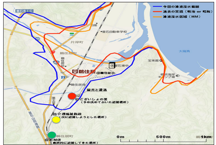
Figure 23. Evacuation and inundation map of Unosumai Town near Kamaishi. The orange line shows the evacuation area, the red line is the approximate inundation from the 1896 and 1933 tsunamis, and the blue line is the 2011 inundation (source: Mainichi Newspaper).
