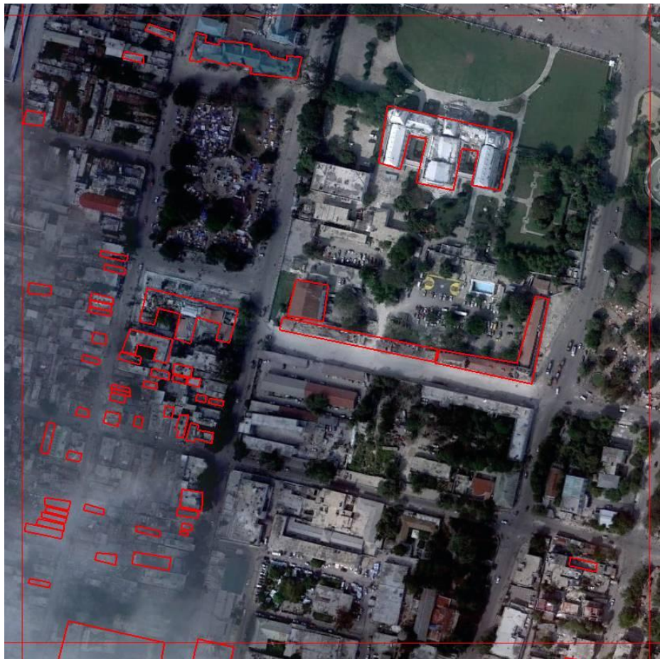
Figure 2: Building footprints for heavily damaged and collapsed structures
